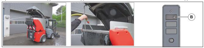
Raise the dirt hopper approx. 50 % with the tip switch (B) so that the water and dirt can be tipped out. Clean the entire dirt hopper from the inside.
