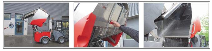
Top up some circulating water and check the circulating water system. Water must reach the suction mouth. Raise the sweeping unit with the joystick (D). Open the rainwater drain valve (option) and check for proper functioning. Clean the vehicle from the outside.
